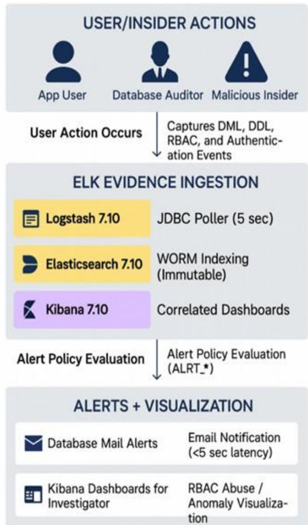
Fig. 3. Forensic audit framework (system architecture).
