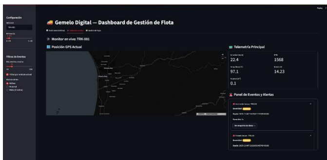
Fig. 3. Digital Twin-based fleet monitoring dashboard showing live GPS position, key telemetry indicators, and active safety alerts.
