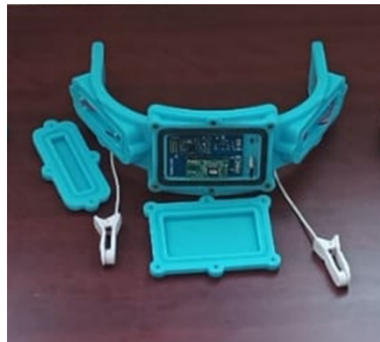
Fig. 12. Electroencephalographic device 3D design: printed with hard resin.
