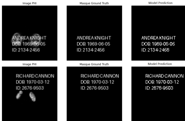
Fig. 2. Detection performance at Epoch 97. The pipeline correctly identifies multi-line PHI blocks (left), generates ground-truth aligned masks (middle), and produces model predictions (right) with high structural fidelity. Note the suppression of low-confidence artifacts in the model predictions.
