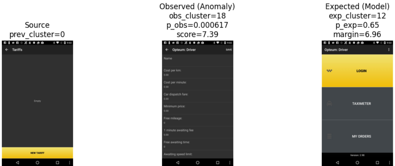
Fig. 6. Detected configuration flow anomaly. From a tariff configuration screen (left), the application navigates to a driver settings page without authentication (middle). The model instead predicts a login screen as the expected continuation (right).
