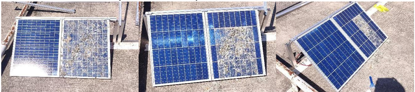
Fig. 3. Photos of the two PV panels with different levels of dirtiness.
