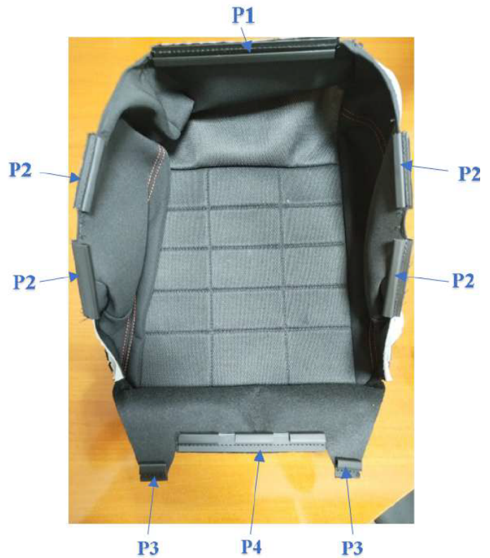
Fig. 1. Automotive seat cover showing J-shaped plastic retainers at different attachment points (P1-P4) that secure fabric to metal frame.
