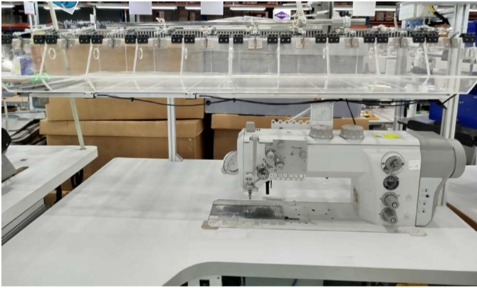
Fig. 2. Current manual assembly workstation showing sewing machine with non-ergonomic component placement requiring repetitive operator reaching.
