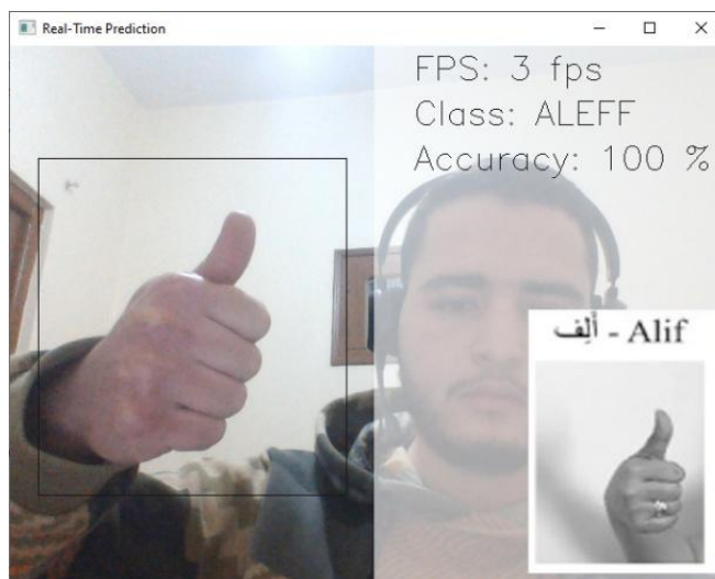
Fig. 11. Real-time gesture recognition prototype built with OpenCV.
