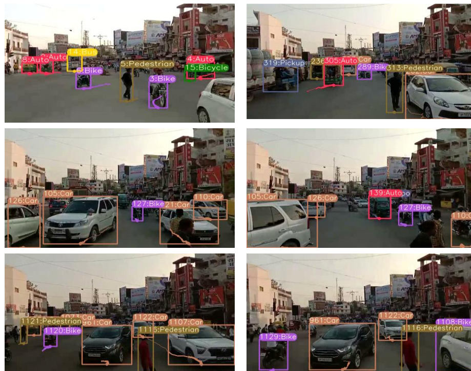
Fig. 8. Detection, localization and multi-class tracking results of the HETRA model under real-world traffic conditions.
