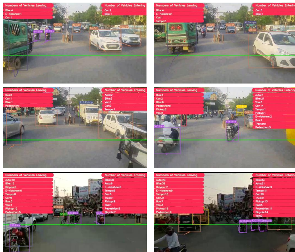
Fig. 9. Directionally classified traffic volume by the HETRA model in real time under heterogeneous traffic conditions.
