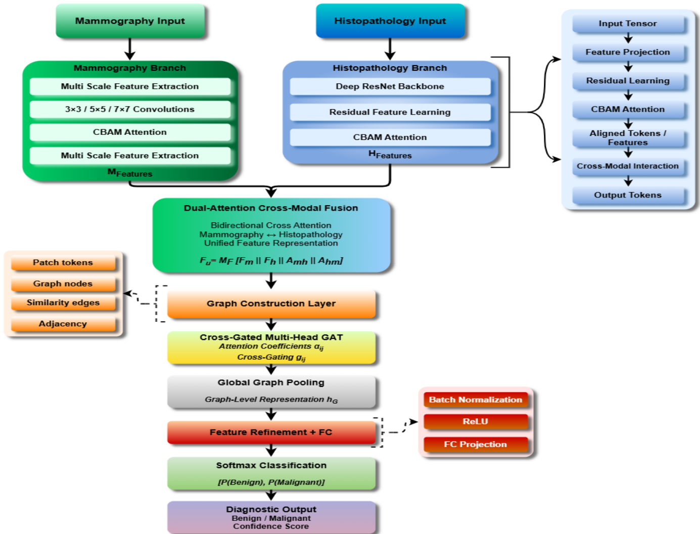
Fig. 3. Proposed MAMGAT-Net architecture for breast cancer diagnosis using dual-stream feature extraction, cross-modal fusion, graph attention learning, and Softmax-based benign or malignant classification.
