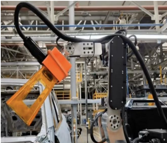
Fig. 1. Vision-guided robot equipped with an electromagnetic marking device.
