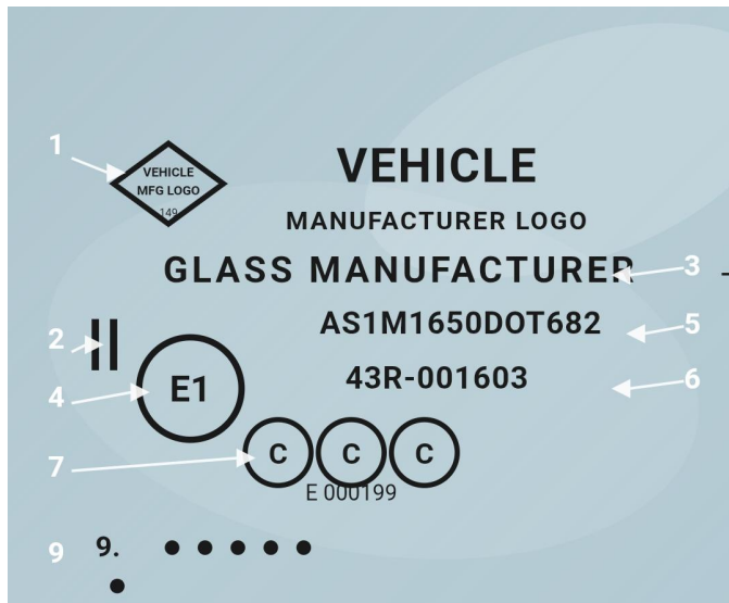
Fig. 1. Regulatory marking elements on an automotive windscreen.
