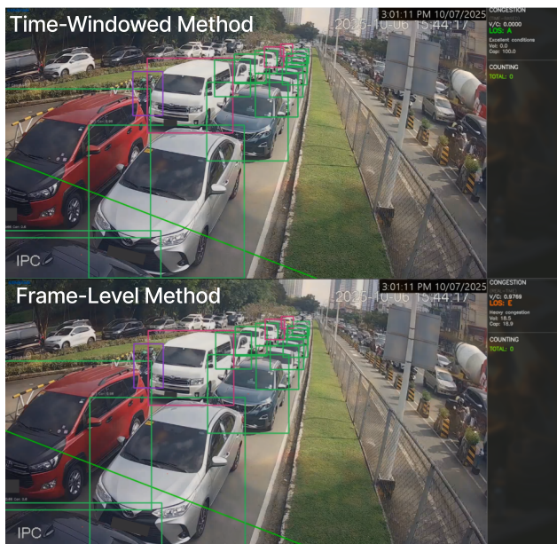
Fig. 7. Time-windowed method (top) vs. frame-level method (bottom) detection comparison in congested states.
