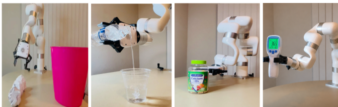
Fig. 11. Assisted robot Arm cleaning area, pouring water, delivering medicine, taking body temperature.
