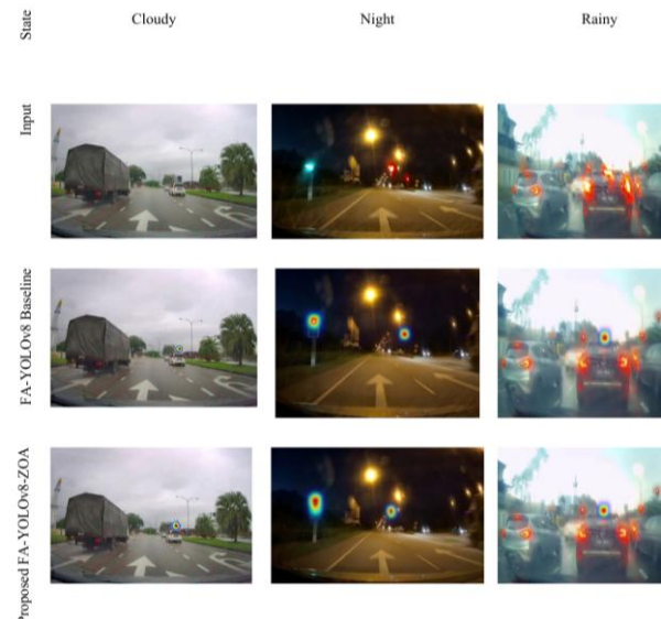
Fig. 4. Representative inputs, baseline FA-YOLOv8 outputs, and proposed FA-YOLOv8-ZOA outputs for cloudy, night, and rainy scenes.
