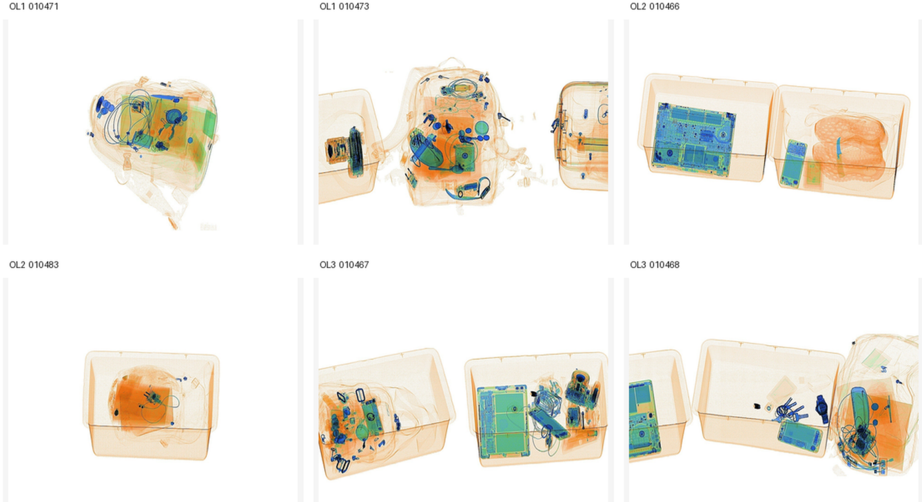
Fig. 4. Representative OPIXray examples from OL1, OL2, and OL3 occlusion-level subsets. The images show the transparent appearance, weak texture, and object overlap that motivate contour-motivated and recall-oriented detection analysis.
