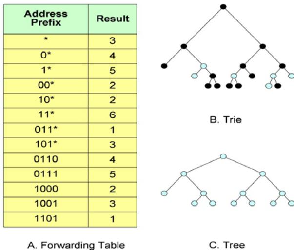
Fig. 3. Trie and tree representations of a forwarding table. In this example, memory consumption of tree is more than trie
