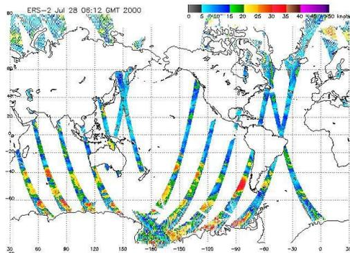
Fig. 8. Example of scatterometer observed ocean wind along with satellite orbit.
