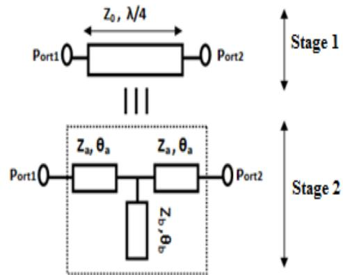
Fig. 6. Equivalent quarter-wavelength transmission line of the T-model
