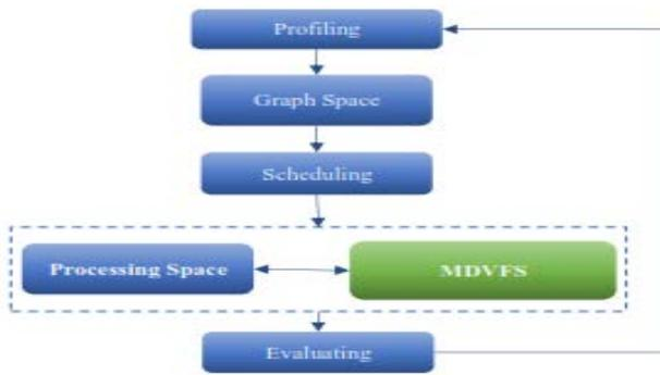
Fig. 2. Internal Work Flow of Storm.
