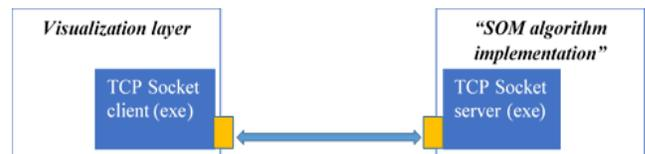
Fig. 7. Placement of TCP Socket Server and TCP Socket Client in Modules.
