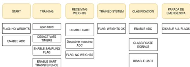
Fig. 4. Finite Machine State Implementation.
