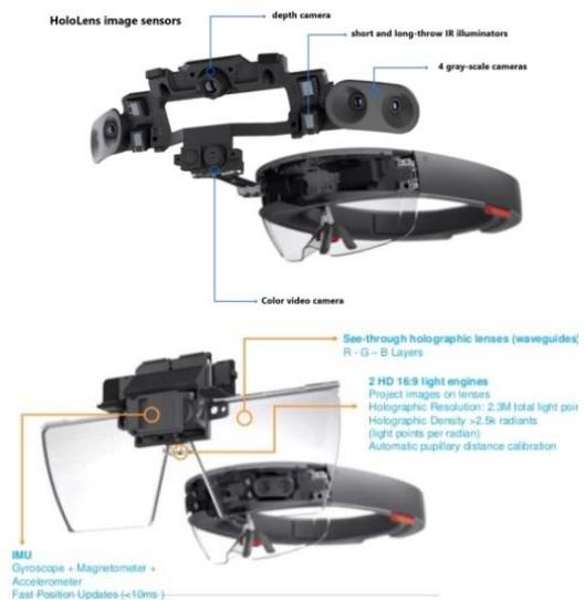
Fig. 1. Sensors on the HOLOLENS.
