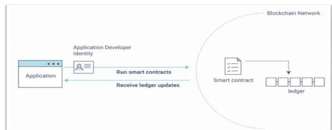
Fig. 1. Interactions in the IBM Blockchain Network.
