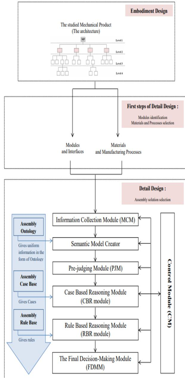
Fig. 1. The Global Structure of the Proposed Automated System for Assembly Solution Selection.
