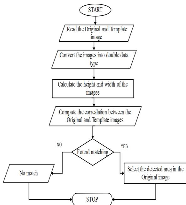
Fig. 3. Flow Diagram of Simple Template Matching.
