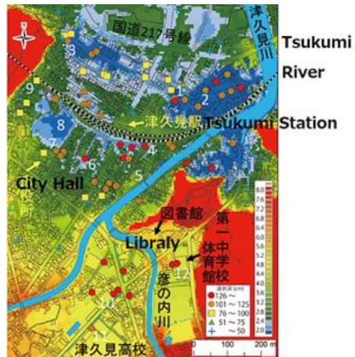
Fig. 5. Flooding Areas in the Tsukumi City Due to Typhoon No.18 (From Journal of Japanese Society on Natural Disaster Science, 36 -4 381 -397 (2018) by Haruhiko YAMAMOTO, Toshiaki YAMASAKI, Kyoko SAKAMOTO and Nao YAMASHITA, Characteristics of Heavy Rainfall and Flood Disaster in Central Southern part of Oita Prefecture by Typhoon No.18 “Typhoon Talim” in 2017).
