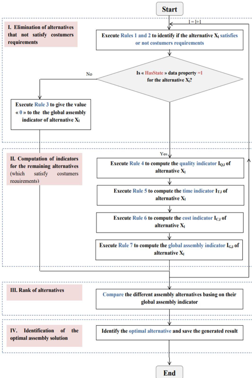
Fig. 6. The Proposed RBR based Decision-Making Process for Optimal Assembly Solution Selection for each Module of the Studied Mechanical Product.
