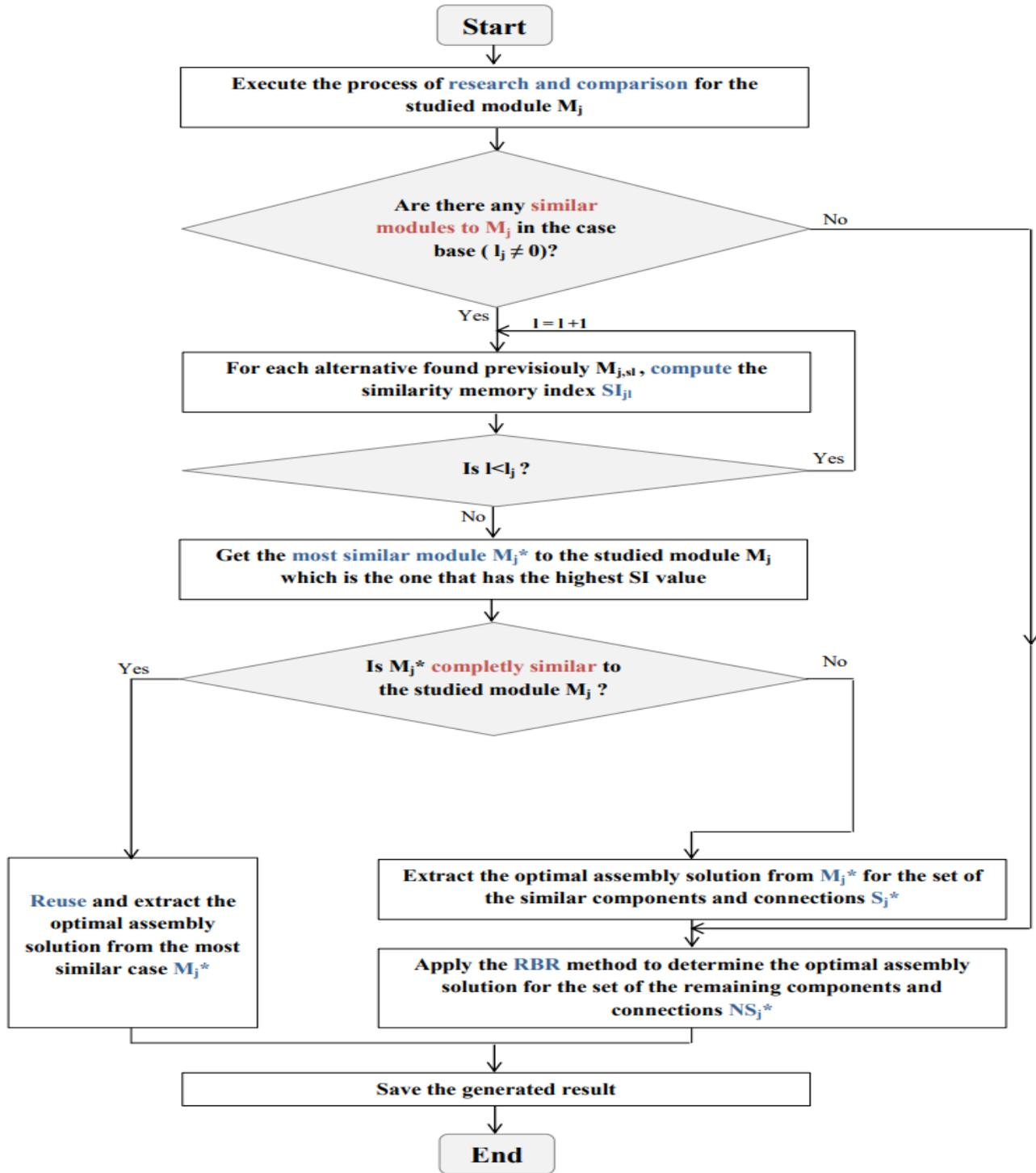
Fig. 5. The Proposed CBR based Decision-Making Process for Optimal Assembly Solution Selection.
