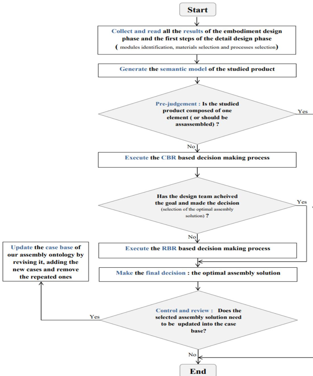
Fig. 2. The Working Process of the ADM System.
