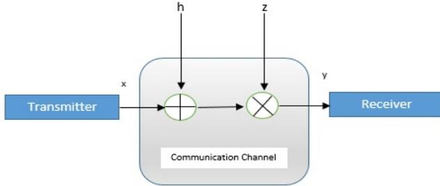
Fig. 1. System Model for Nakagami-q Fading SISO Wireless Channel.
