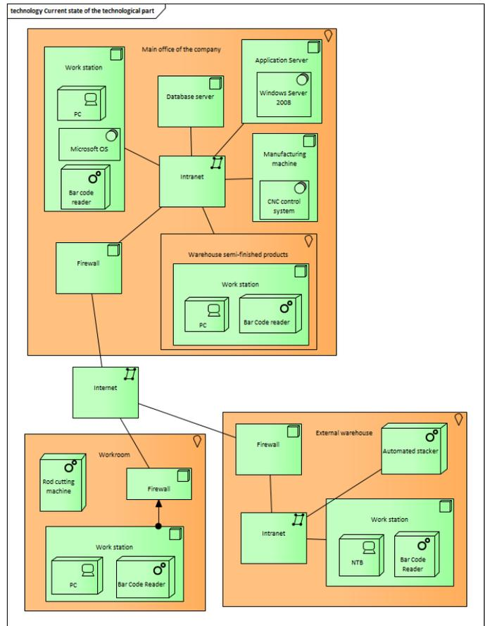
Fig. 13. Current State of the Technological Part
