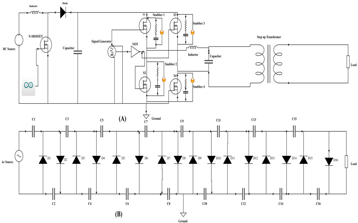
Fig. 7. Complete Circuitry of Power Supply (A) Boost Converter and Inverter (B) Cockcroft Multiplier
