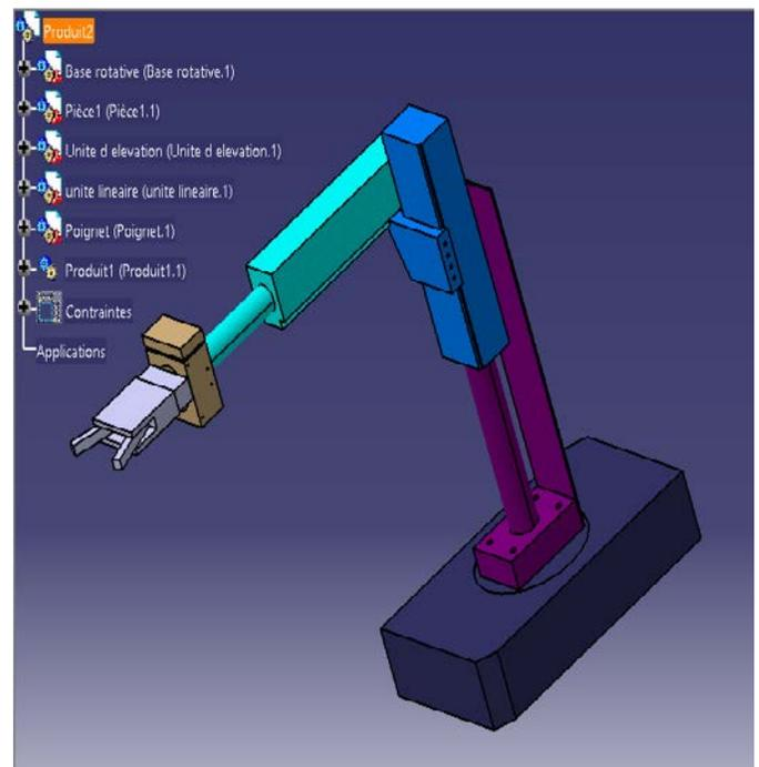
Fig. 7. The Schrader Robot Architecture: Its Different Modules.
