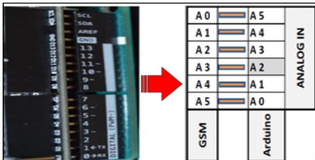
Fig 6. Connect GSM to the Arduino ANALOG IN.
