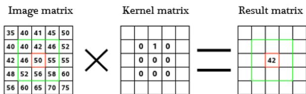
Fig. 3. Image Matrix Convolution Process with a Kernel Matrix.
