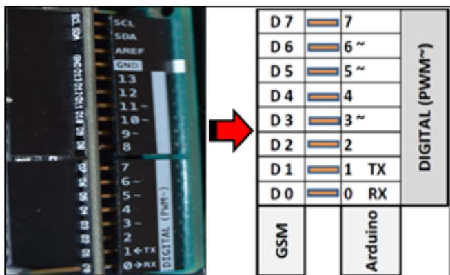
Fig 5. Connection between GSM and Arduino DIGITAL (PWM~).
