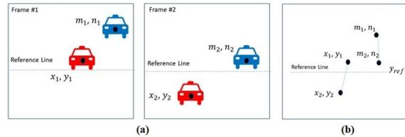
Fig. 4. (a) Sample Images from Two Consequent Frames, i.e. Frame#1 and Frame#2. (b) The Vehicle is Tracked from the Minimum Displacement from the First Frame to the Second Frame.
