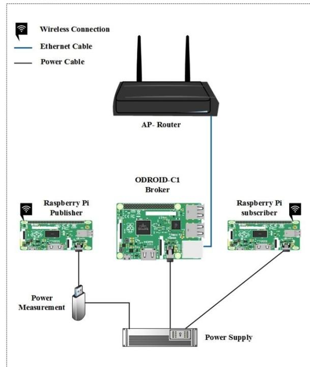
Fig. 1. General Test Environment Architecture.
