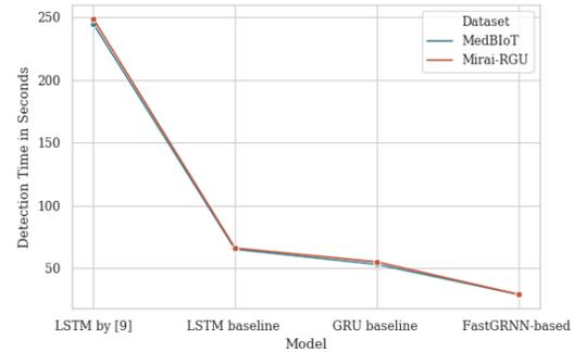
Fig. 9. The Required Detection Time of The Proposed FastGRNN-based Model Compared to Other Models.
