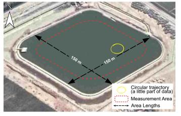
Fig. 9. Measurement Area of the Agricultural Water Reservoir with Dimensions and Circular Trajectory of the Unmanned Vehicle.
