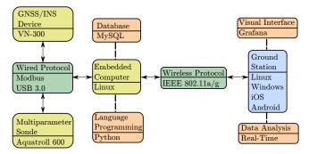
Fig. 2. Block Diagram of the Water Quality Measurement System.
