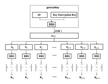
Fig. 3. Sub-keys Generator in Decryption Process.
