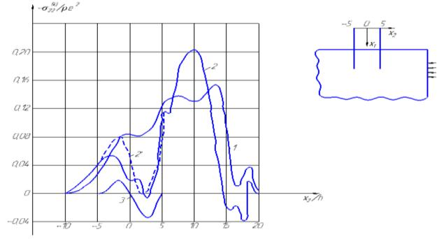
Fig. 5. Change of Normal Stresses  $\sigma_{22}^k$  at Time t=60 $\tau$  along the  $x_2$  Coordinate in Sections  $1 - x_1 = 5h$ ,  $2 - x_2 = 10h$ ,  $2' - x_1 = 10h$ ,  $3 - x_1 = 0h$ .
