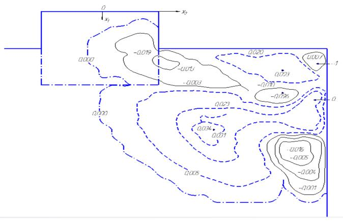
Fig. 6. Tangential Stress Isolines  $\sigma_{12}^k$  (k = 1,2) at Time t=40 $\tau$ .
