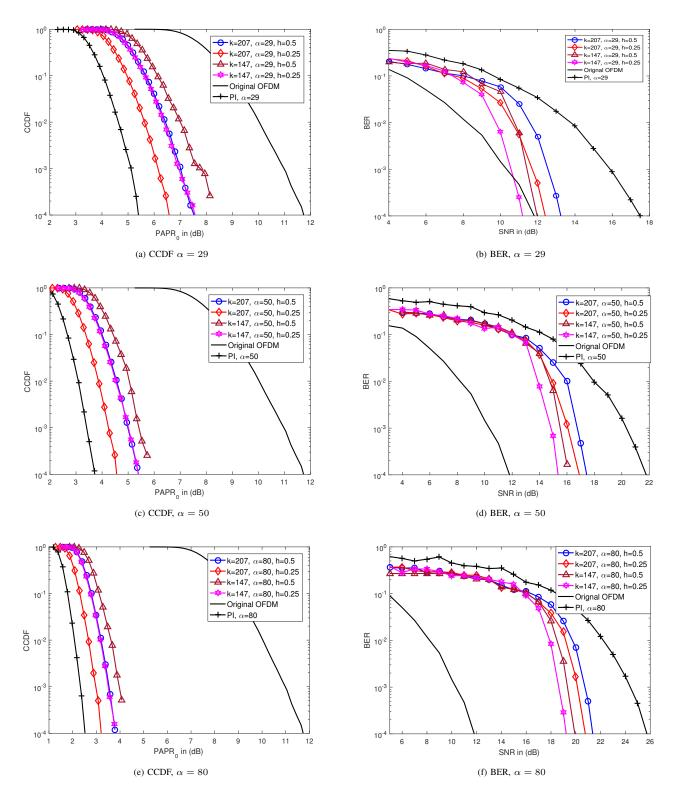
Fig. 7. CCDF and BER Performances of the proposed BCB-OFDM Compared with Peak Insertion and Normal OFDM, NFFT=256 with QAM Modulation Versus  $\alpha$ .
