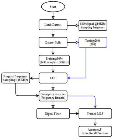
Fig. 18. Illustration of the Process Flow of the MLP for AC Fault Classification.
