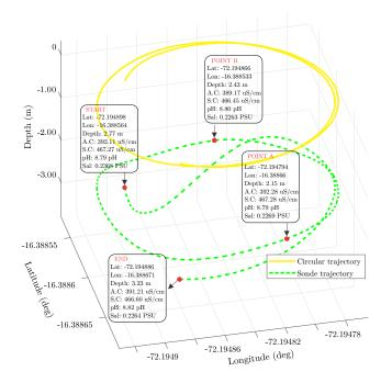
Fig. 10. Water Quality Measurement with Accurate Global Positioning in Underwater Space Environment (Lat: Latitude; Lon: Longitude; Depth; A.C: Actual Conductivity; S.C: Specific Conductivity; pH: Potential of Hydrogen; Sal: Salinity).
