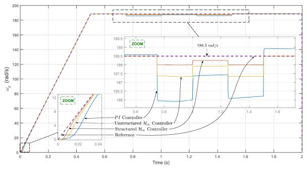
Fig. 9. Controlled Variable Comparison, Rotor Speed  $\omega_r$ .
