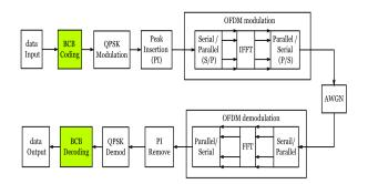
Fig. 2. BCB Peak Insertion in OFDM Systems.
