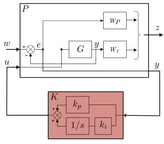
Fig. 2. Structured  $\mathcal{H}_{\infty}$  Controller.
