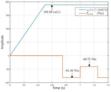
Fig. 6. Reference Speed  $\omega_r(ref)$  and Mechanical Torque  $T_{mech}$ .
