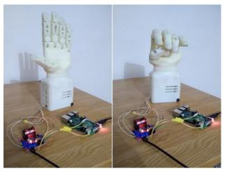
Fig. 6. Control of the Prosthetic 3D Printed Hand.
