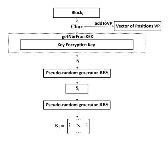
Fig. 2. Sub-keys Generator in Encryption Process.
