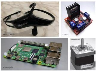
Fig. 2. Hardware Components.
