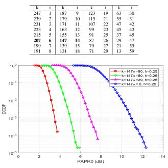
Fig. 3. CCDF Curves of the Proposed BCB-OFDM NFFT=256, 4QAM,  $BCB(n = 255, k = 147, v = 64, \alpha)$  with Variable  $\alpha$ .
