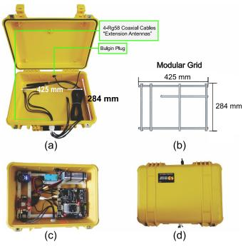
Fig. 7. Case Dimensions with Modular Grid for Supporting Embedded Computer and Electronics.
