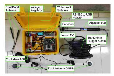
Fig. 6. Hardware Architecture of the Water Quality Measurement System.
