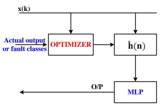
Fig. 15. Synchronization of Frequency Domain Bandpass Digital Filter with MLP.
