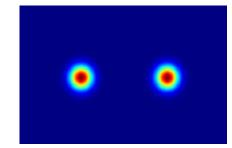
Fig. 1. Thermal Distribution of Two Heat Sources as Picked up by an Array Sensor after Interpolation.
