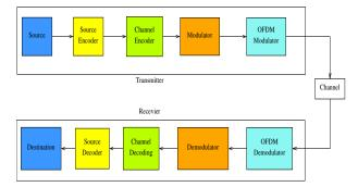
Fig. 1. Communication Digital Systems Block with OFDM.
