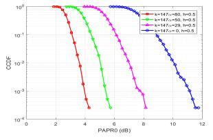
Fig. 5. CCDF Curves of the Proposed BCB-OFDM NFFT=256, 4QAM,  $BCB(n=255,k=147,v=128,\alpha) \text{ with Variable } \alpha.$
