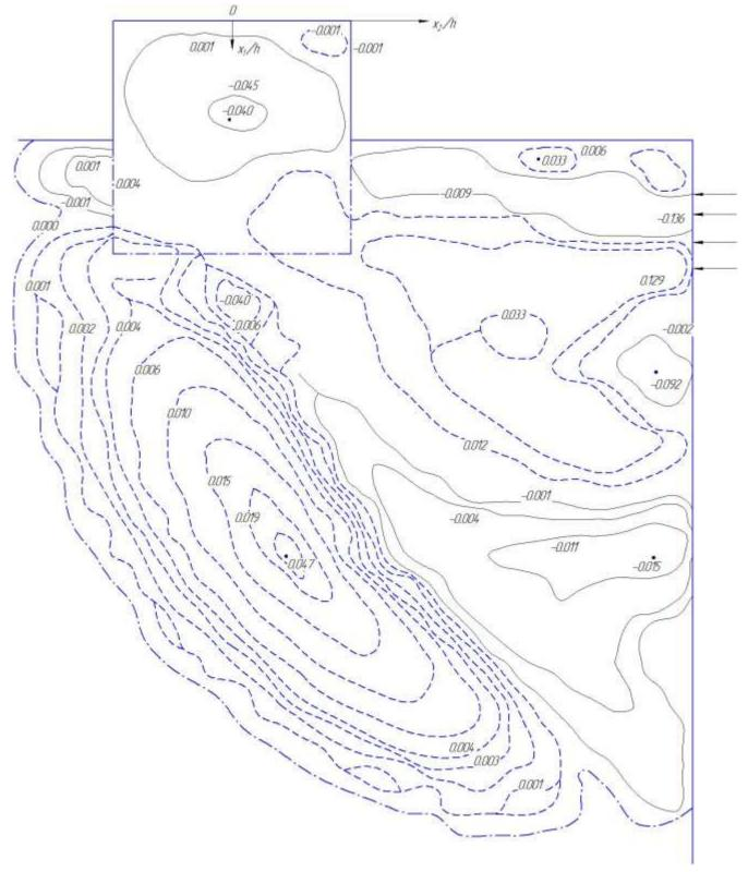
Fig. 7. Tangential Stress Isolines  $\sigma_{12}^k$  (k = 1,2) at Time t=60 $\tau$ .
