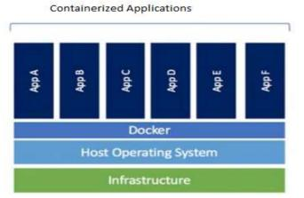
Fig. 2. Containerized Applications on Single OS through Docker.
