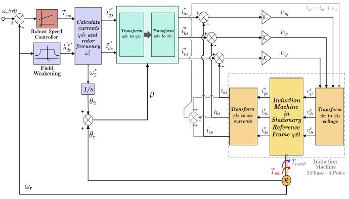
Fig. 3. Simulator of Induction Motor in Simulink.
