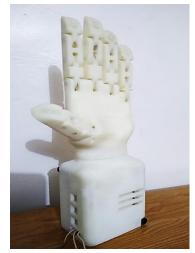
Fig. 3. Prototype of the Prosthetic Hand.
