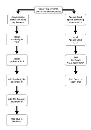
Fig. 2. The Experimental Environment Setup.
