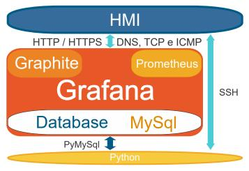
Fig. 4. Software Architecture of the Proposed System.
