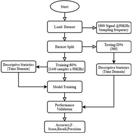
Fig. 12. Illustration of the Process Flow of the LSTM for AC Fault Classification.
