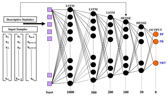
Fig. 10. LSTM Model for AC Fault Classification.
