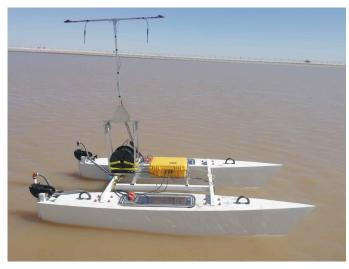
Fig. 8. System Carried on an Unmanned Surface Vehicle in a Water Quality Measurement Mission of a Huge Agriculture Reservoir.
