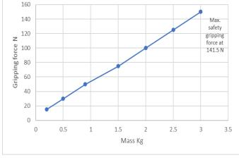
Fig. 7. Maximum Gripping Force and Weight.
