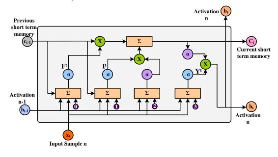
Fig. 9. Basic Structure of LSTM Cell.
