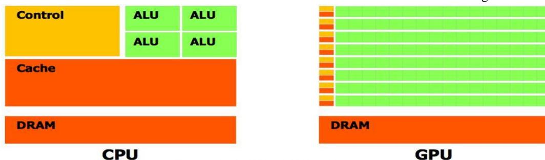
Figure 1: Basic CPU and GPU Architecture
