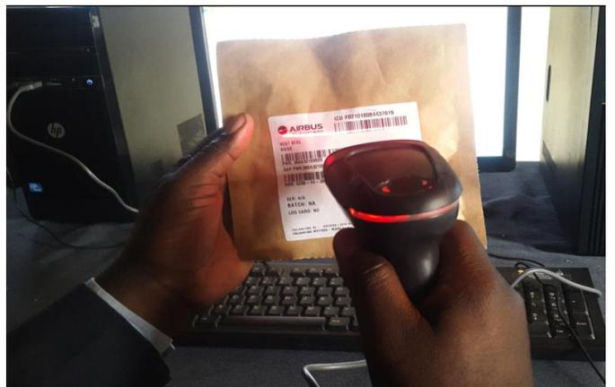
Fig. 15. Adding spares by using barcode reader.
