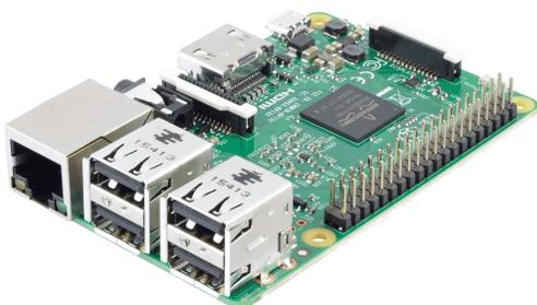
Fig. 1. Raspberry Pi 3 embedded system.
