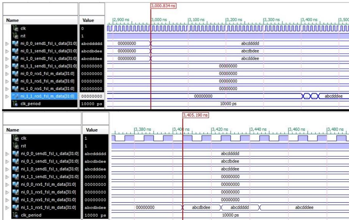
Fig. 8. Simulation waveform during packet transmission in 2x2 2D-mesh topology.
