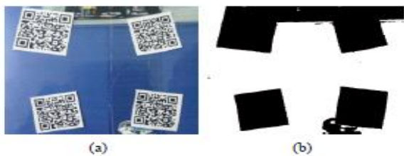
Fig. 4. Regions of interest extraction. (a) Original image. (b) Resulting binary mask in which the black areas refer to the regions of interest which may contain QR code.
