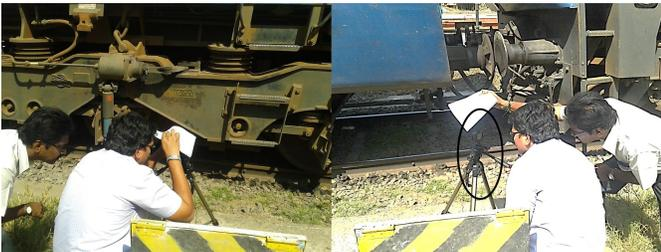
Fig. 3. Train Bogie Video Recording using High Speed Sports action Camera.
