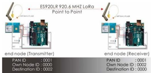
Fig. 7. Pairing ES920LR LoRa use Arduino board (Design\_1).
