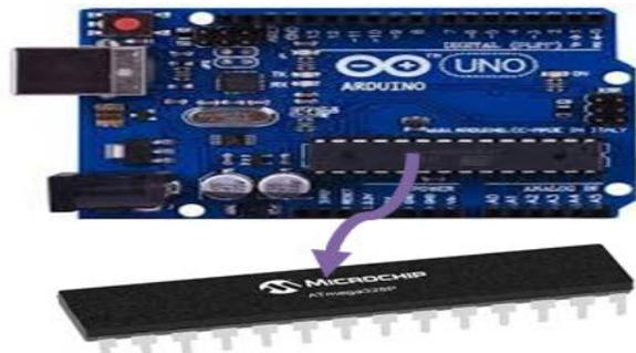
Fig 5. Arduino Uno with ATmega328P Microcontroller.
