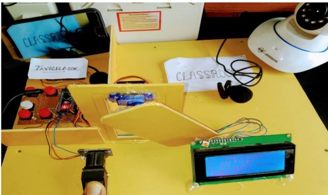
Fig 17. Opening Door Shows Successful Authentication.
