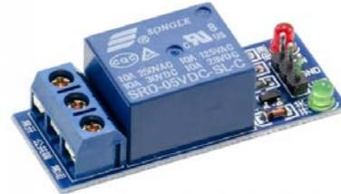
Fig. 7. Single Channel 5V Relay Board.
