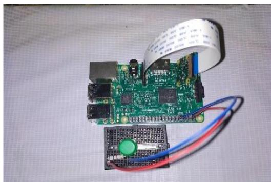
Fig. 5. System Setup after Connecting Hardware Components.
