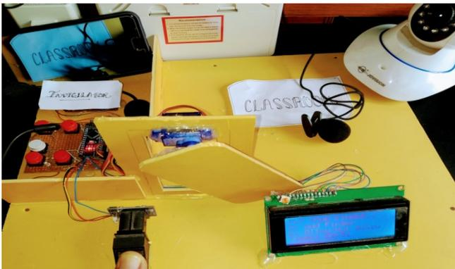
Fig 17. Opening Door Shows Successful Authentication.
