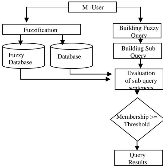
Figure 5: The Block diagram of the fuzzy tool
