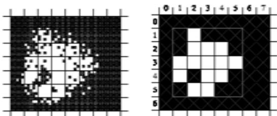
Fig. 3. (a) An example of  $S_{ij}$  (b) Noise removal by the  $5 \times 5$  filter
