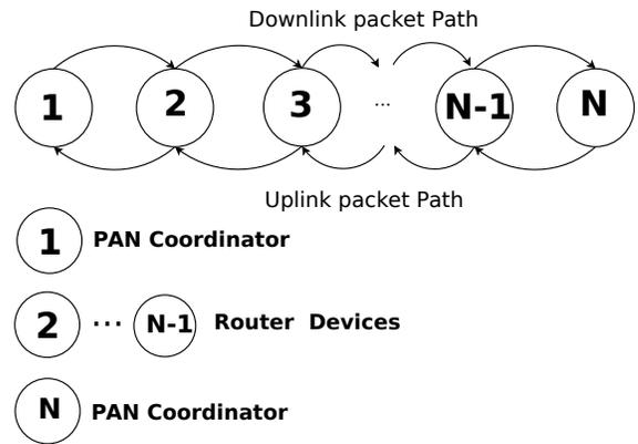
Fig. 2: LWSN Topology and type of network devices
