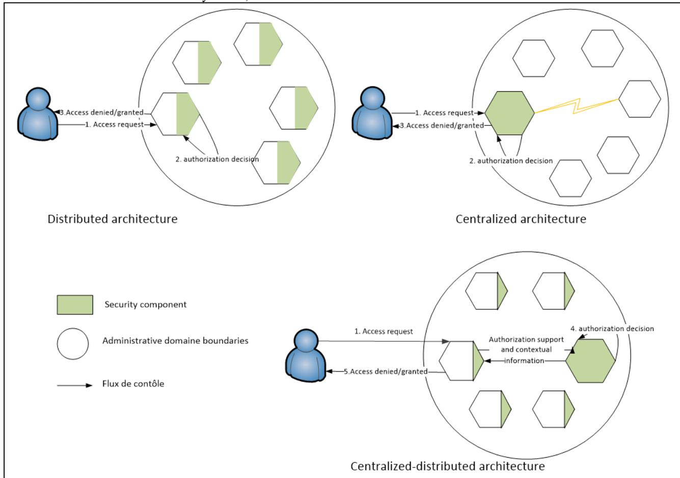
Fig. 1. Main architectures for IoT access control
