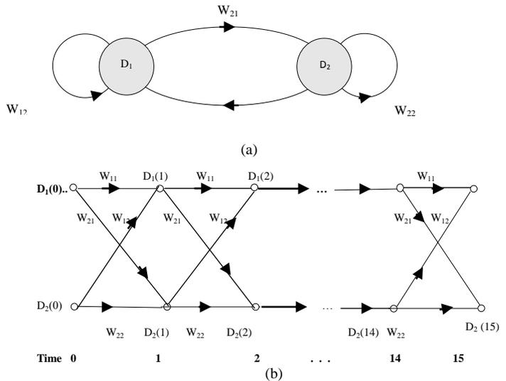
Fig. 5. Back Propagation Through Time model (a) Architecture Graph of two neurons and (b) Single flow graph of network 15 unfolded in time
