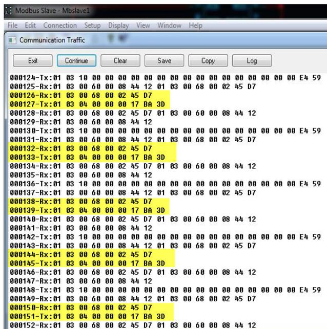
Fig. 15. Modbus Slave Communication Log
