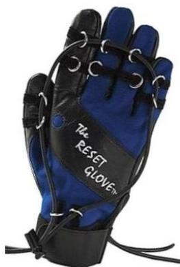
Fig. 2. Resistive interface glove [18]
