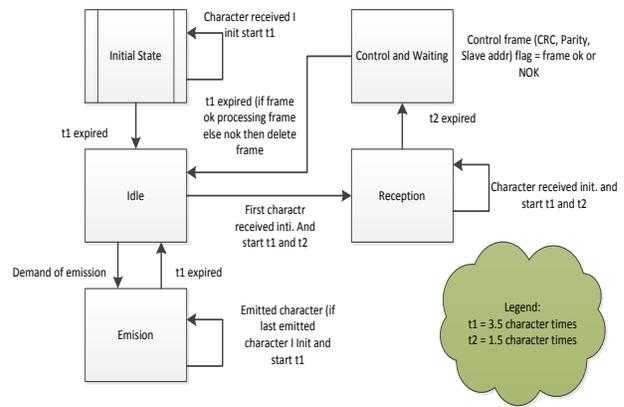
Fig. 11. Modbus Master Transmission Mode State Diagram
