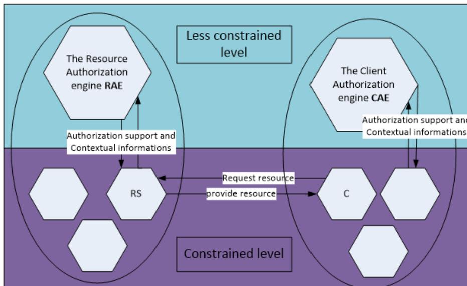
Fig. 2. Constrained and less constrained layers
