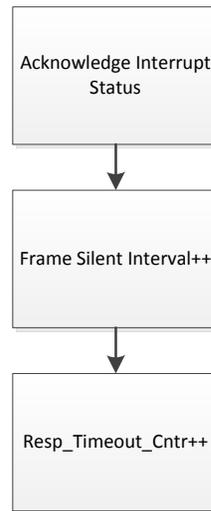
Fig. 8. Timer 2 (250usec) – Interrupt Service Routine
