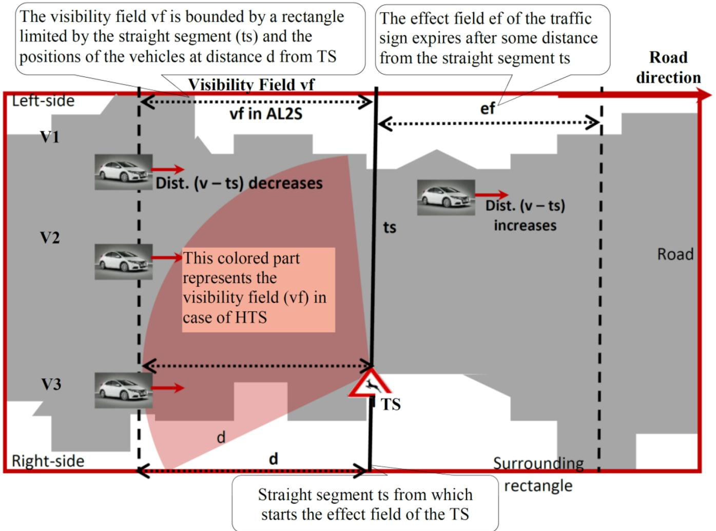
Fig. 7: TS as a plan. The road and a TS projected into a two dimensions space. The road is colored in grey, the vf of the HTS is colored in orange and vf of the soft TS (in AL-S<sup>2</sup>m) is indicated by a discontinuous arrow.
