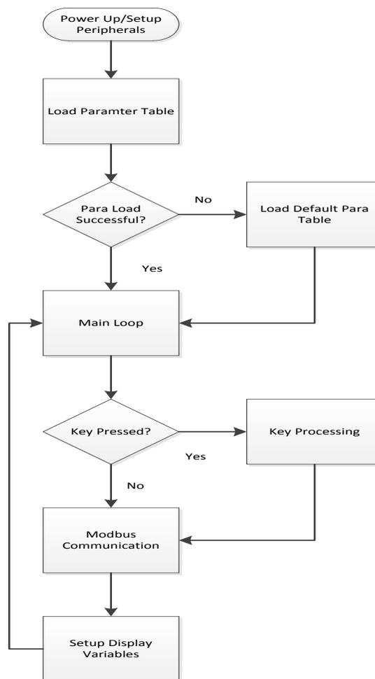
Fig. 6. Operator Panel Interface Main Call Graph
