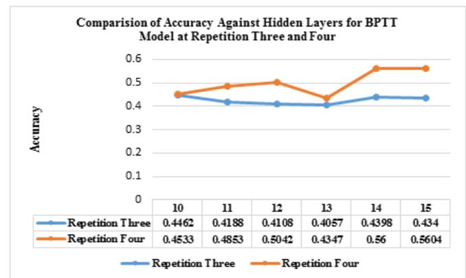
Fig. 7. Comparison of the accuracy versus the hidden layers for the BPTT model with repetitions of three and four
