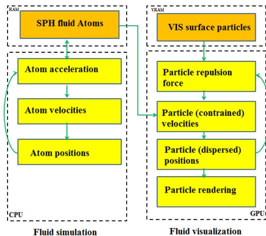
Fig. 2: Surface visualization on GPU
