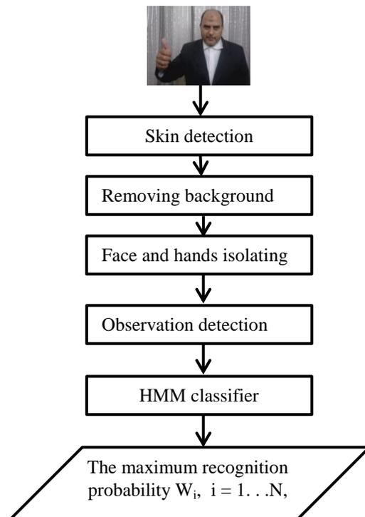
Fig. 2. Proposed system architecture
