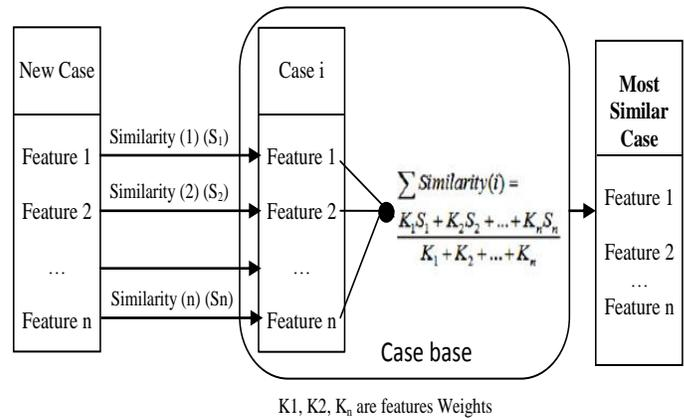
Fig. 2. the retrieval mechanism of CBR
