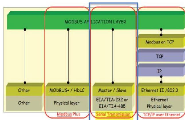
Fig. 4. Modbus and the OSI Layer
