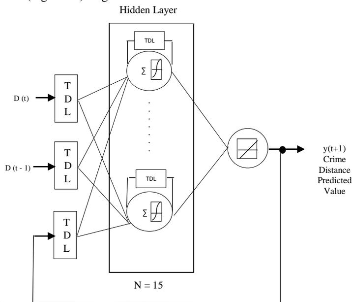
Fig. 4. Nonlinear autoregressive NARX model with exogenous inputs
