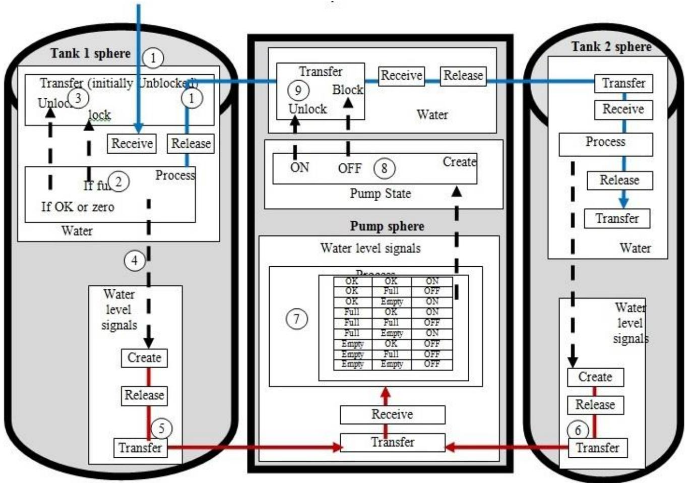
Fig. 3. FM representation of the pumping control system
