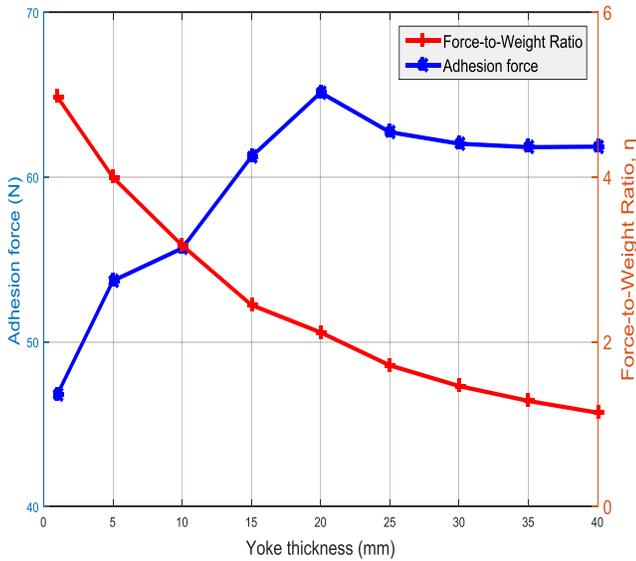
Fig. 11. Adhesion force for yokes with different thicknesses
