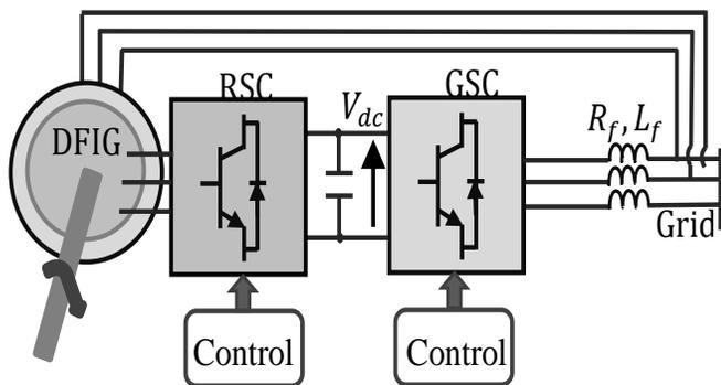
Fig. 1. Bloc diagram of WECS connected to the grid
