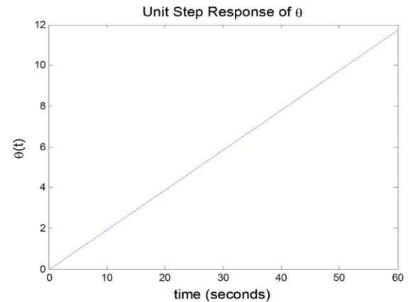
Fig. 10. Unit step response of beam angle  $\theta$
