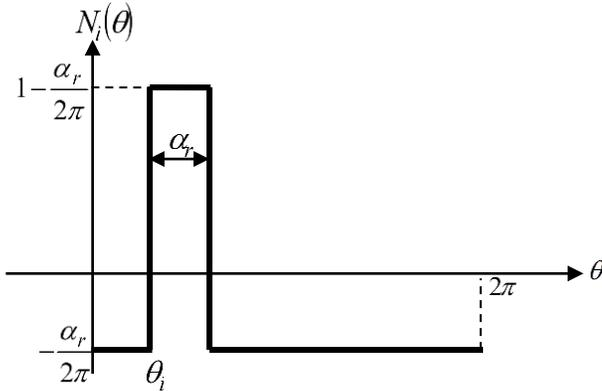
Fig. 1. Rotor loop winding function of healthy generator
