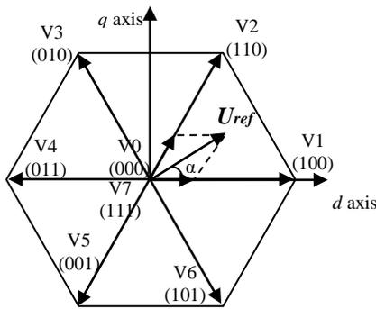
Fig. 5. Basic switching vectors and sectors
