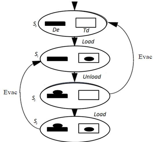
Fig. 1: Kripke Structure of parts conveying robot
