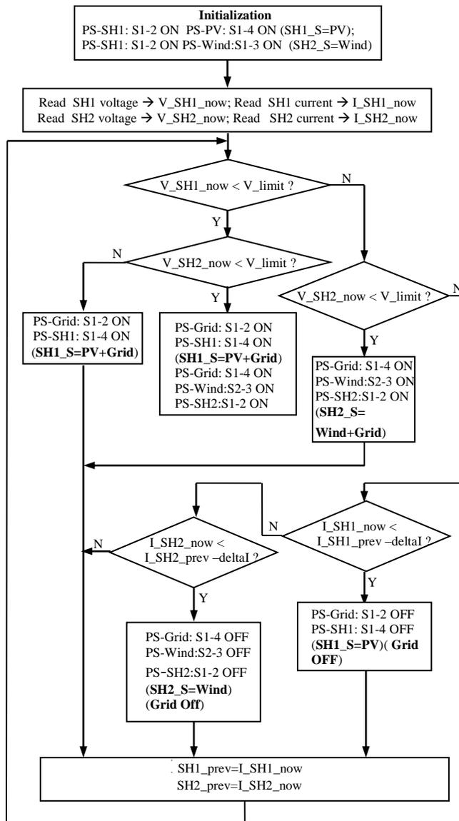
Fig. 6. Flowchart of the continuous supply algorithm
