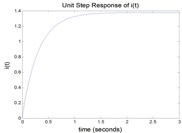
Fig. 13. Unit step response of armature current  $i_a(t)$
