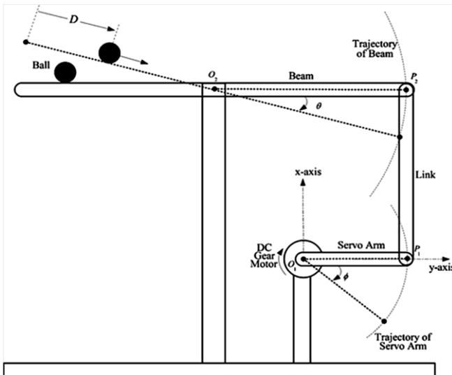
Fig. 2. Functional description of the hardware platform
