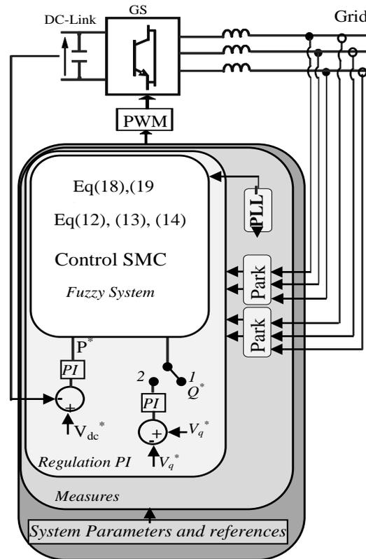
Fig. 6. Bloc diagram of WECS connected to the grid
