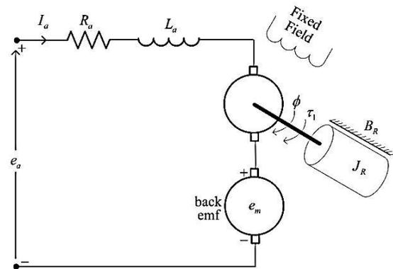
Fig. 3. Electrical and mechanical modeling diagram of PMDC motor
