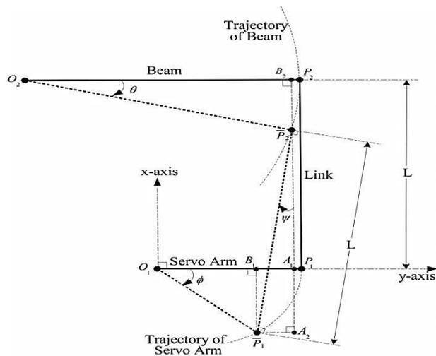
Fig. 5. Geometrical description of the hardware platform
