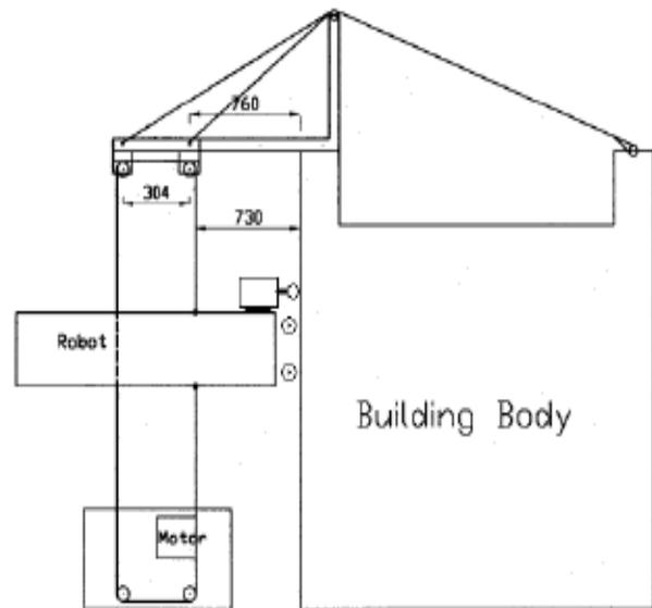
Fig. 2. Block diagram of Tile-Wall robot system [13]
