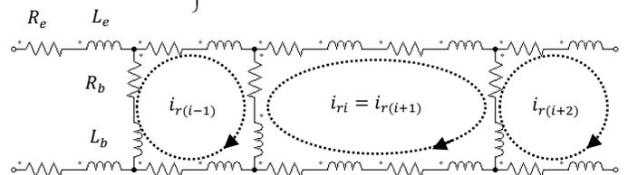
Fig. 3. Equivalent circuits of a squirrel cage rotor with one broken bar
