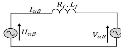
Fig. 2. Equivalent circuit of VSC in stationary frame
