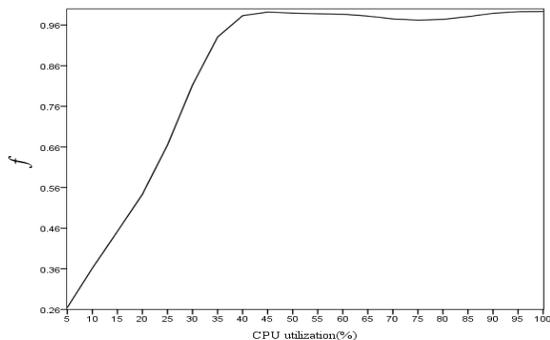
Fig. 5. Corresponding relationship curve between the CPU utilization and the operating frequency
