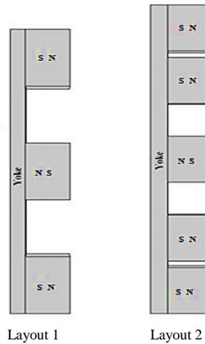
Fig. 13. Proposed N-S-N and N-N-S-N-N magnet arrangement layouts
