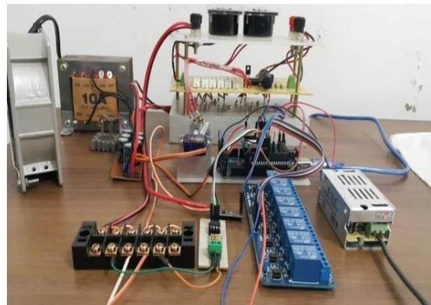
Fig. 12. PV simulator hardware.
