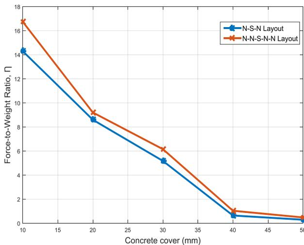
Fig. 16. Force to weight graph for two layouts
