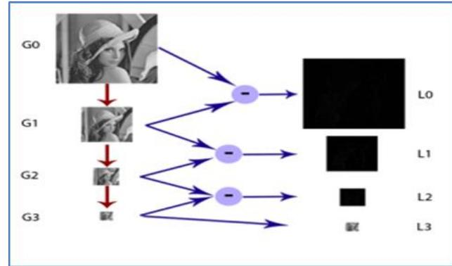
Fig. 1. The construction of the Laplacian pyramid for the Lena image [20]
