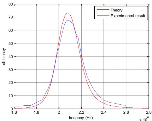
Fig. 6. Efficiency versus frequency at 15.5cm distance and  $f_0 = 2.07\text{MHz}$  (Mutual Inductance Effect)
