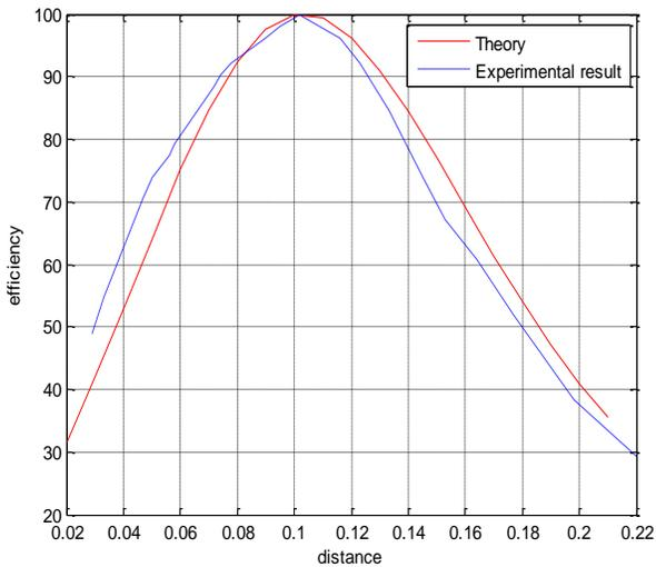
Fig. 10. Efficiency versus distance at resonant frequency
