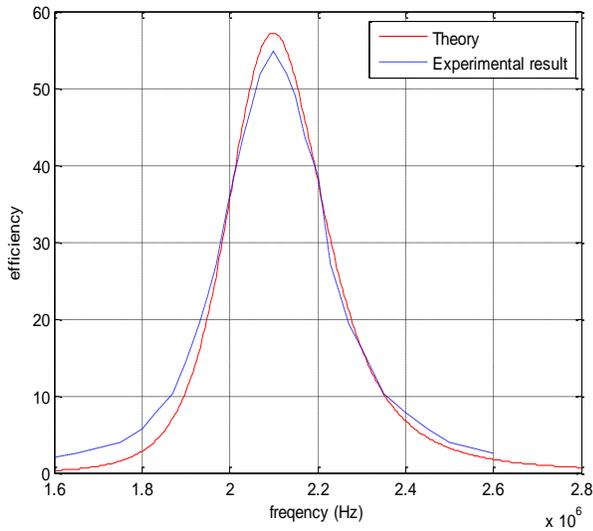
Fig. 13. Efficiency versus frequency at 3cm distance
