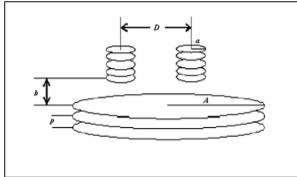
Fig. 3. Schematic Circuit of a Resonant coupled system
