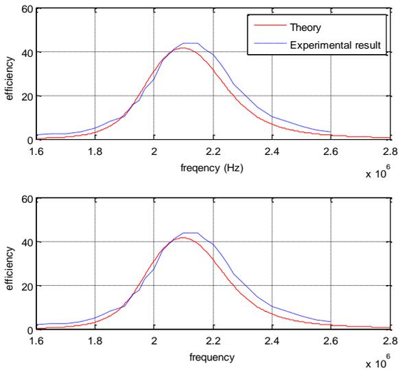
Fig. 14. Efficiency versus frequency for two receivers system
