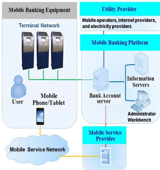
Fig. 2. Mobile Banking System Architecture
