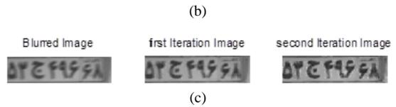
Figure 5. Deblurring LP images using proposed approach
