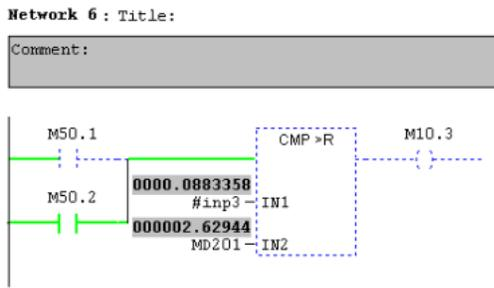
Figure 10. Compare Logic Element (CMP) in FB1
