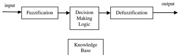
Fig. 4: Fuzzy Controller Block Diagram
