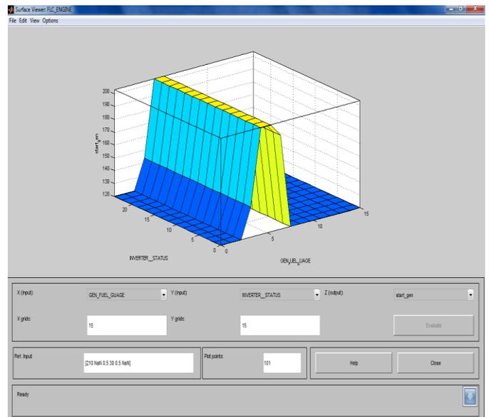
Fig. 6.6: ICOFLS surface viewer Results for the process fuel gauge, inverter status and Control variable start-gen.
