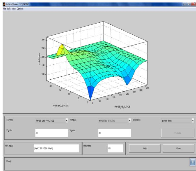
Fig. 6.9: ICOFLS surface viewer plots for the process variable (Inverter Status, phase voltage) control variable (switch lines).
