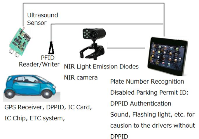
Fig. 2. System configuration of the proposed DPP system
