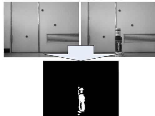
Fig. 6. Background subtraction method, left-top is background image and right-top is current image. Background subtraction method will obtain black-white image (bottom)
