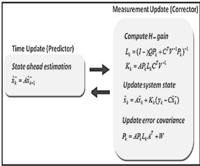
Fig. 10. The process flow of the H<sup>∞</sup> filter algorithm
