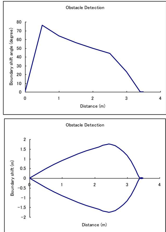
Fig. 12. measuring obstacle avoidance performances
