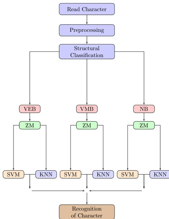
Figure 3. Block Diagram of Proposed Character Recognition System
