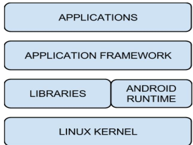
Fig. 1. The Android Architecture
