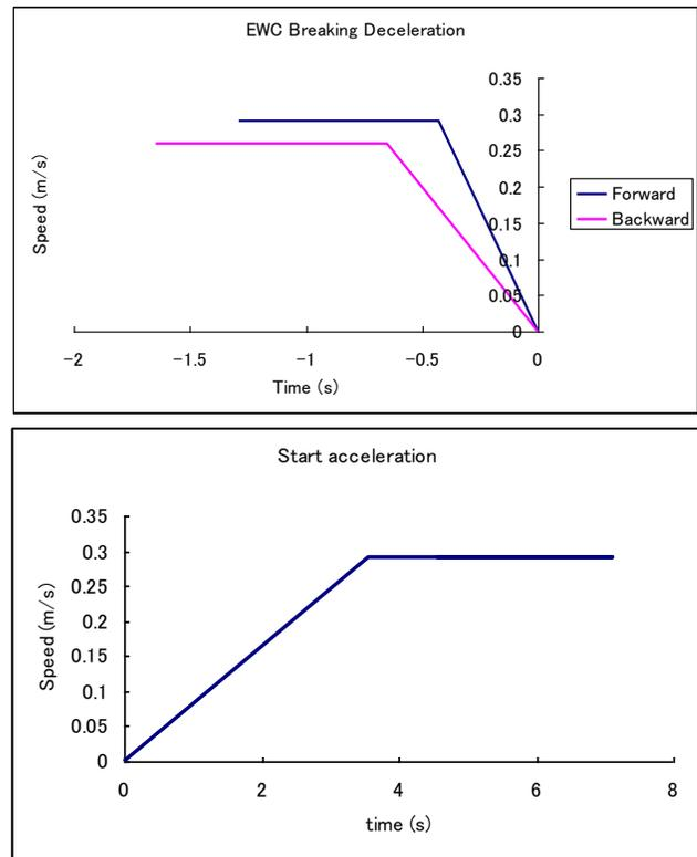
Fig. 15. Experiment of EWC acceleration and deceleration
