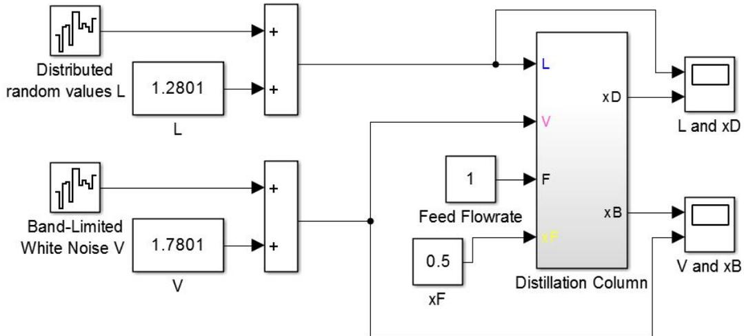
Fig. 3: MATLAB/Simulink model of the distillation column
