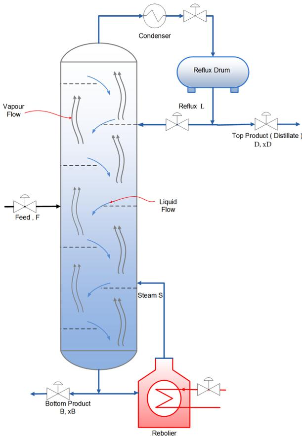
Fig. 1: Schematic diagram of a binary distillation column
