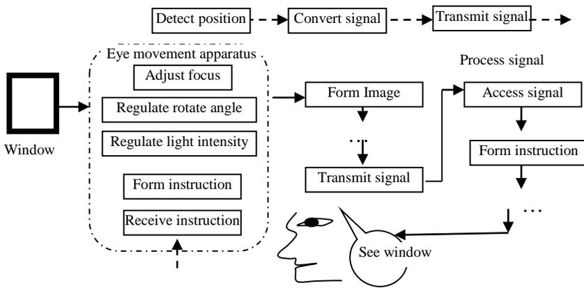
Fig. 2. “Whole flow path of the artificial vision system” (partial figure – re-drawn from Jin Ma et al. [20])
